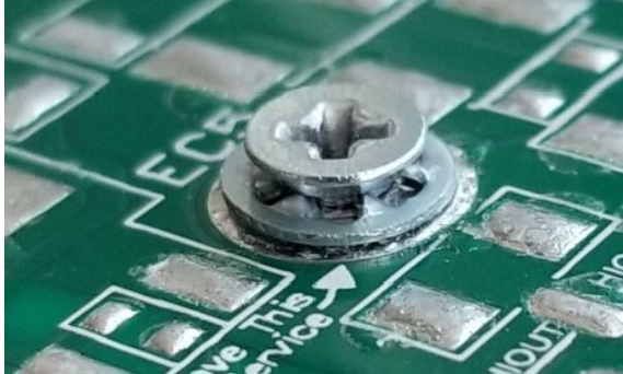
Properly fixed and seated screw and washer
