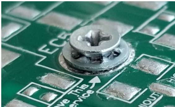
Properly installed and seated screw and washer
