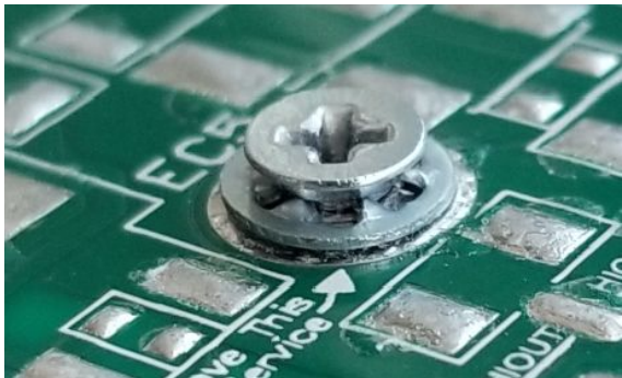
Properly fixed and seated screw and washer
