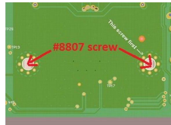
Dip each screw in Loctite. Counter 2 threads.
