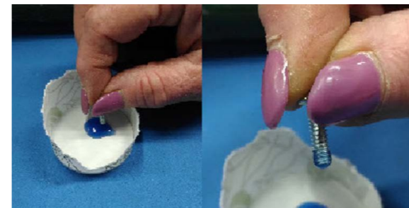
7 Mount 6698 using 2 #8807 screws. Dip the screws in Loctite. Tighten to 4 in lbs.
