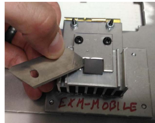
4 Place the 4236 pad onto the heatsin. Handle the 4236 pad by the edges only.
