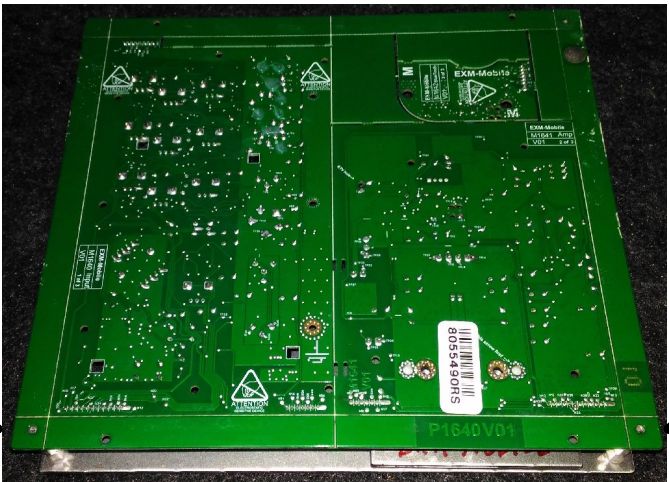
6) Place M1639 face down on the jig. Pin at the two lower corners.
