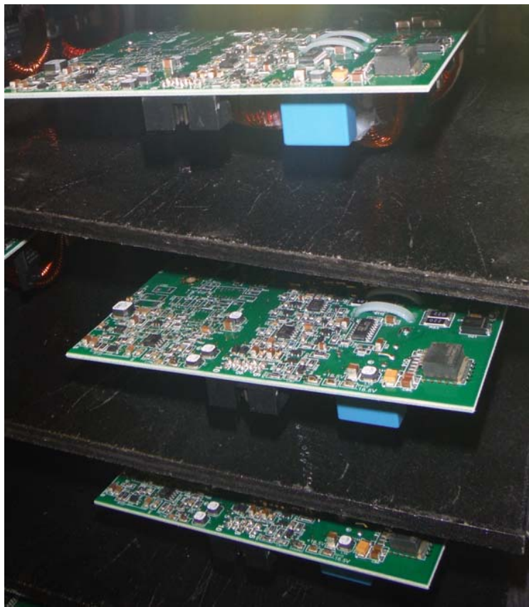
BOARDS PLACED UPSIDE DOWN ON RACK AFTER WAVE SOLDERING
